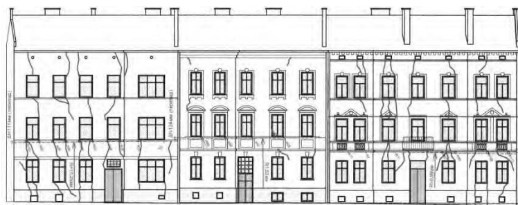
Fig. 4. Picture of crack formations on the main facade of the group of residential buildings of old buildings located in Lviv in Pid Dubom Str.
