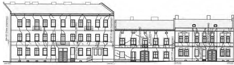
Fig. 6. Picture of crack formations on the main facade of the group of residential buildings of old buildings located in Lviv inth Dzherelna Str.
